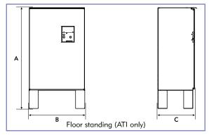
$<sup>^{\</sup>star} Floor$  standing.  $^{\dagger} Dimension$  A for the top cable entry model will change to 1350 mm (53.1 in)
